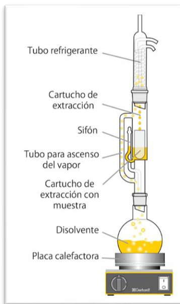
Figura 5. Partes del extractor Soxhlet
